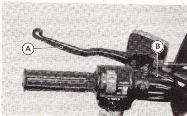
A. Clutch Lever B. Starter Lockout Switch
